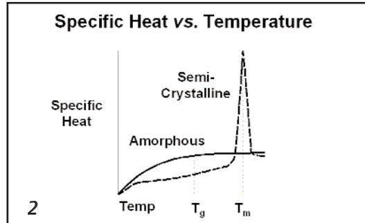
They have a broad softening temperature ( $T_g$ , glass transition temperature) range (Figure 2) that allows the material to soften gradually, melt and flow without prematurely solidifying. These polymers generally are very efficient with regard to their ability to transmit ultrasonic vibrations, and can be welded under a wide range of force/amplitude combinations.
